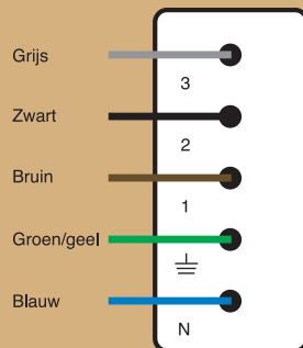
Codering 5-polige chassisdelen
