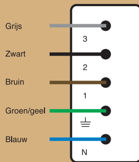
Codering 5-polige chassisdelen
